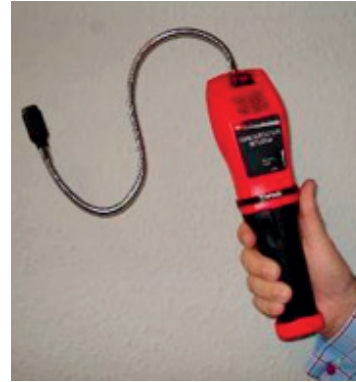
Figure 3 - Electronic leak detectors suitable for flammable refrigerants
